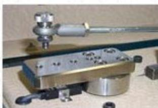
The linear motion arm has an adjustable stroke length, variable to accommodate virtually any required contact surface area of a test specimen. The precision bearing on the splined shaft allows the abrading head to 'float', freely following the specimen surface whether contoured, irregular, or flat.
