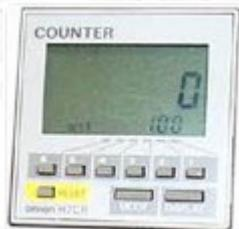
The test counter is programmable from 1–999,999 test cycles. It features an LCD back lit display for improved visibility.
