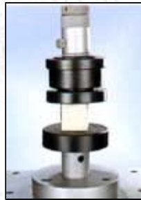
SF122 Bending Fixture
